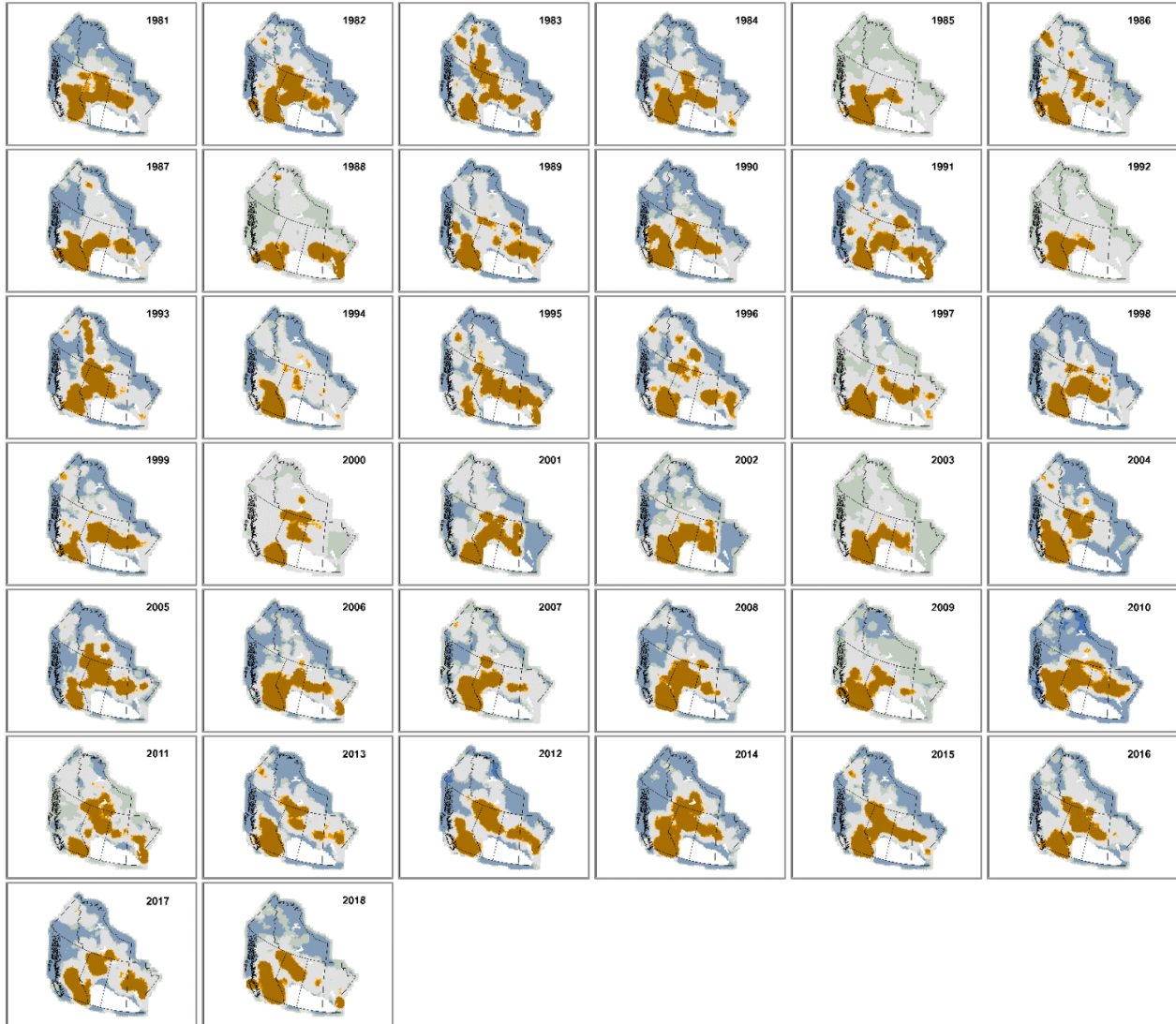
Figure 3.5: Getis-ord statistic computed for lightning-ignited wildfires for Western Canada by year, 1981-2018. Each graph is represented by its z-score for significance, where orange denotes significant positive z-scores at 90, 95 and 99% confidence intervals. Gray indicates no significant z-score, blue signifies significant negative z-scores at 90, 95, and 99% confidence intervals and white indicates that it was excluded from the analysis.
