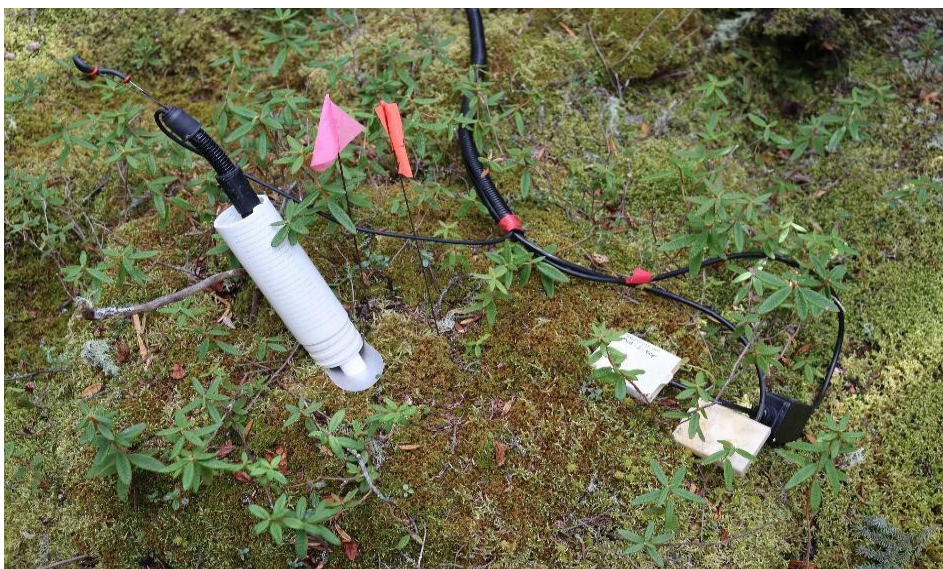
Image 4. Plot setup at Pelican Mountain with tensiometer and moisture probes for measuring peat moisture dynamics.
